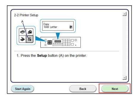
Carefully follow the instruction to select **Wireless LAN setup** on the printer. Press the **OK** button on the printer. Then , click **Next** on the **Printer Setup** (2-3) screen.
