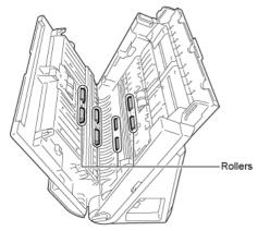
5 Remove the retard roller and feed roller. (See "Replacing the Feed Roller" on p.96, "Replacing the Retard Roller" on p.97)
