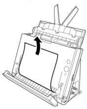
4 Return the document eject tray to its original position. Make sure that it is completely closed by pushing until you hear a click.
