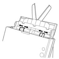
3 Place the card horizontally with the top edge facing upward.
