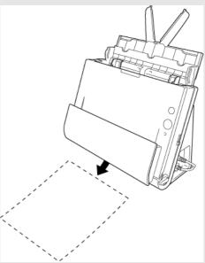
When scanning multiple page documents that are fastened together, such as invoices, place the documents so that the edge that is fastened together is facing down.
