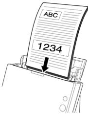
After inserting the document in the document feeder, align the document guides with both edges of the document.
