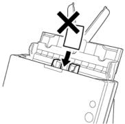
Ultrasonic double feed detection will not function properly when scanning cards. Clear the [Detect by Ultrasonic] check box in the [Feeding] tab.
