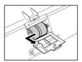
3 Install the new feed roller. When installing the feed roller, align the notch on the roller with the shaft of the front unit.
