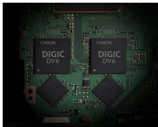
Figure 13 Two DIGIC DV6 processors to implement all video processing prior to encoding for recording
