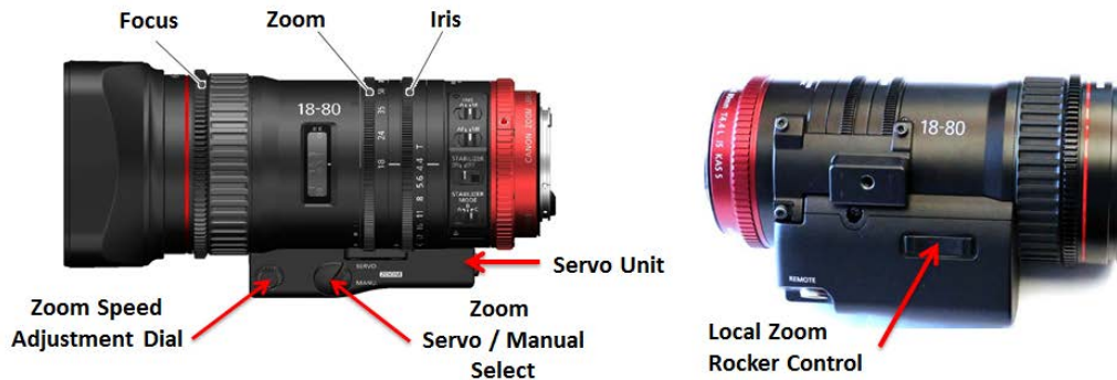
Figure 7 Integral zoom servo unit separates the Canon Compact Servo lens from other Compact Lenses
