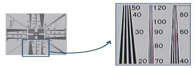
Figure 4 Showing the resolution of the EVF in the vicinity of picture center exceeds 900 TVL/ph
