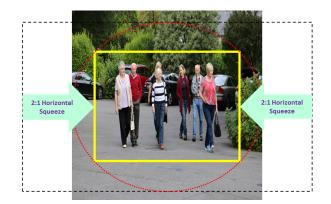
**Figure 13** Showing the 2:1 compressed optical image projected by the anamorphic lens onto the 4:3 aspect ratio S35mm film format or the 4:3 aspect ratio image sensor of some digital cinema cameras
