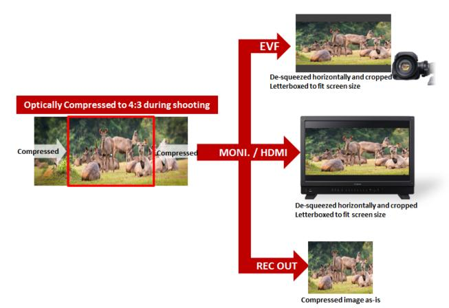
**Figure 17** De-squeeze and letterboxing in the EOS C700 EVF and in the optional DP-V2410 reference display
