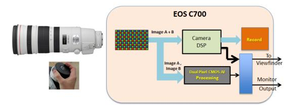
**Figure 11** Showing the Focus Guide mode of operation – that opens the control loop to the lens and instead the data processing sends signaling to the viewfinder and monitor output feed that guides the manual focus action
