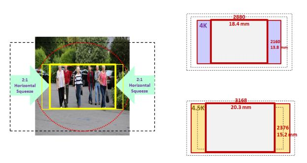
**Figure 16** Showing the active image (heavy yellow rectangle) projected by a 2.0 anamorphic lens on to the EOS C700 Super 35mm image sensor having a 17:9 aspect ratio (DCI specification) and its different dimensions for 4K and 4.5K origination
