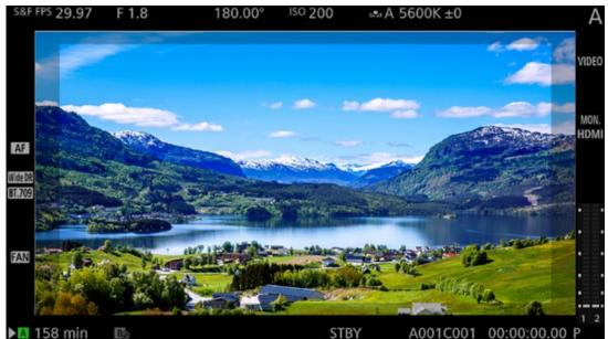
**Figure 5** With DCI viewing angle in record mode, the surround is displayed in letterbox on the 16:9 EVF panel.
