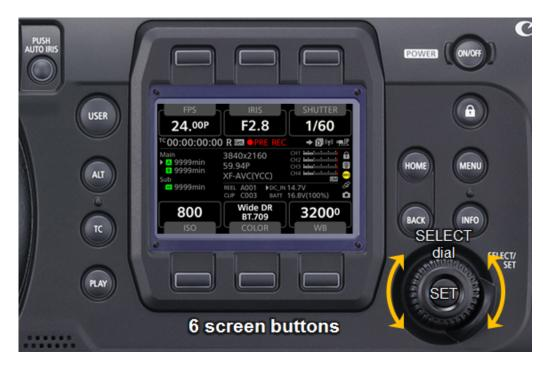
Figure 18The camera operational panel on the left side of the EOS C700
