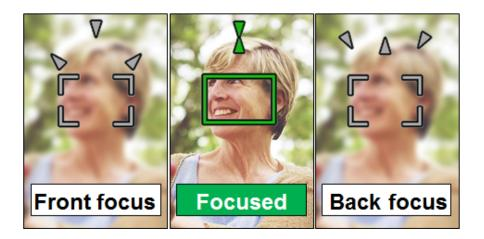
**Figure 10** The focus guide cursor detail uses three arrows to indicate to the camera operator the direction to manually rotate the focus control. At the point of precise focus on the chosen subject the cursor snaps to a green color.
