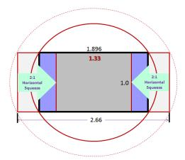
**Figure 15** The anamorphic 2.0 lens compresses a 2.66:1 aspect ratio input optical image to a 1.33: aspect ratio onto the 17:9 image sensor
