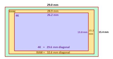
**Figure 2** Showing the relative dimensions of the two image formats – the 4K and the 4.5K RAW
