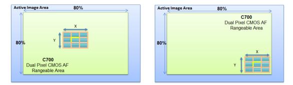
**Figure 8** The Dual Pixel CMOS AF selection area can be moved around 80% of the active image frame to allow selection of different subjects within the scene for sharp focus
