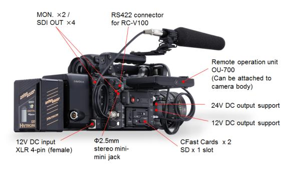
Figure 20Overview of the primary operational interfaces of the EOS C700
