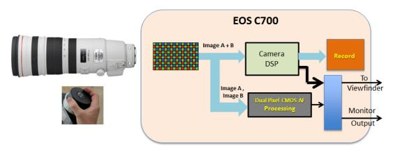
Showing the Focus Guide mode of operation – that opens the control loop to the lens and instead the data processing sends signaling to the viewfinder and monitor output feed that guides the manual focus action
