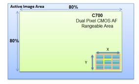
**Figure 8** The Dual Pixel CMOS AF selection area can be moved around 80% of the active image frame to allow selection of different subjects within the scene for sharp focus
