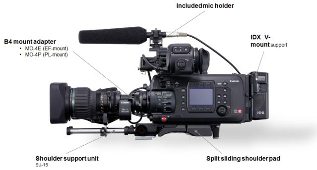
**Figure 25** The C700 offers a choice of between an EF and a PL version of a B4 mount adapter that enables the use of standard 2/3-inch broadcast zoom lenses
