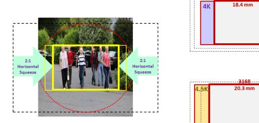
Figure 16 Showing the active image (heavy yellow rectangle) projected by a 2.0 anamorphic lens on to the EOS C700 Super 35mm image sensor having a 17:9 aspect ratio (DCI specification) and its different dimensions for 4K and 4.5K origination
