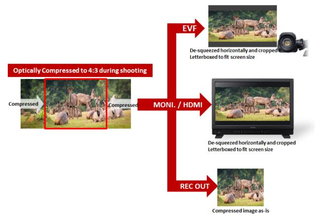
**Figure 17** De-squeeze and letterboxing in the EOS C700 EVF and in the optional DP-V2410 reference display
