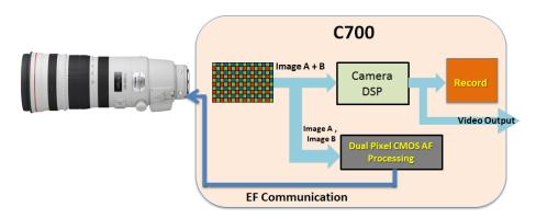
Figure 7 Showing the separate processing of the dual pixel data from the image sensor – for both video and for Auto Focus
