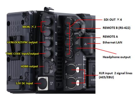
Figure 21 Close-up of the primary system interfaces on the rear of the EOS C700
