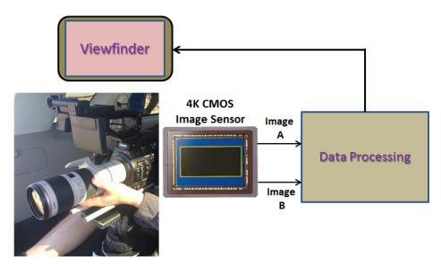
**Figure 9** Principle of the Focus Guide system – where manual actuation of the lens focus control is detected by the image sensor and the data processing signals the viewfinder
