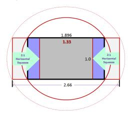
**Figure 15** The anamorphic 2.0 lens compresses a 2.66:1 aspect ratio input optical image to a 1.33: aspect ratio onto the 17:9 image sensor
