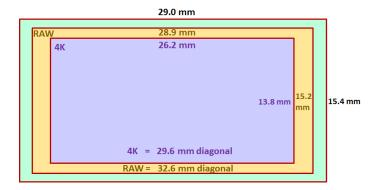
Figure 2 Showing the relative dimensions of the two image formats – the 4K and the 4.5K RAW
