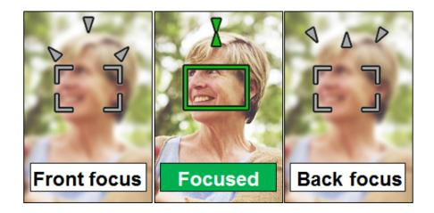
The focus guide cursor detail uses three arrows to indicate to the camera operator the direction to manually rotate the focus control. At the point of precise focus on the chosen subject the cursor snaps to a green color.
