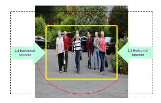
Figure 13 Showing the 2:1 compressed optical image projected by the anamorphic lens onto the 4:3 aspect ratio S35mm film format or the 4:3 aspect ratio image sensor of some digital cinema cameras
