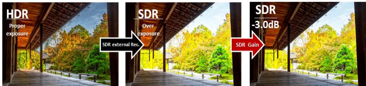
Figure 30 Accurate HDR exposure of a bright outdoor scene will require a decrease in gain to properly set the effective exposure of the associated SDR video being simultaneously recorded
