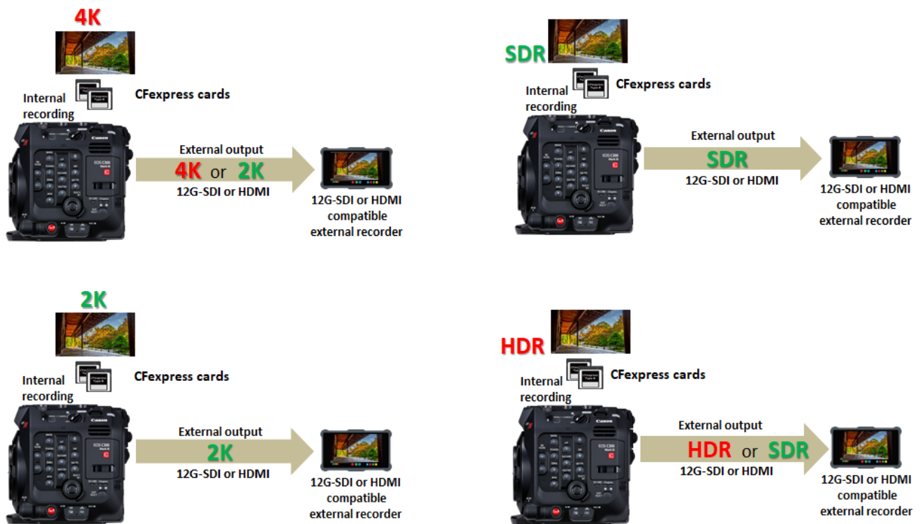
Figure 32 Allowable combinations of on-board and external recording of HDR / SDR and 4K / 2K
