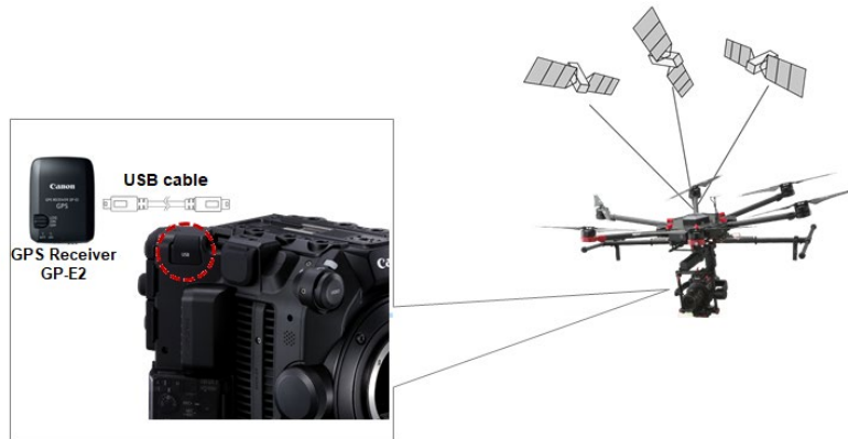
Figure 61 A GPS receiver can simply connect to the USB port on the EOS C300 Mark III and provide location and time information
