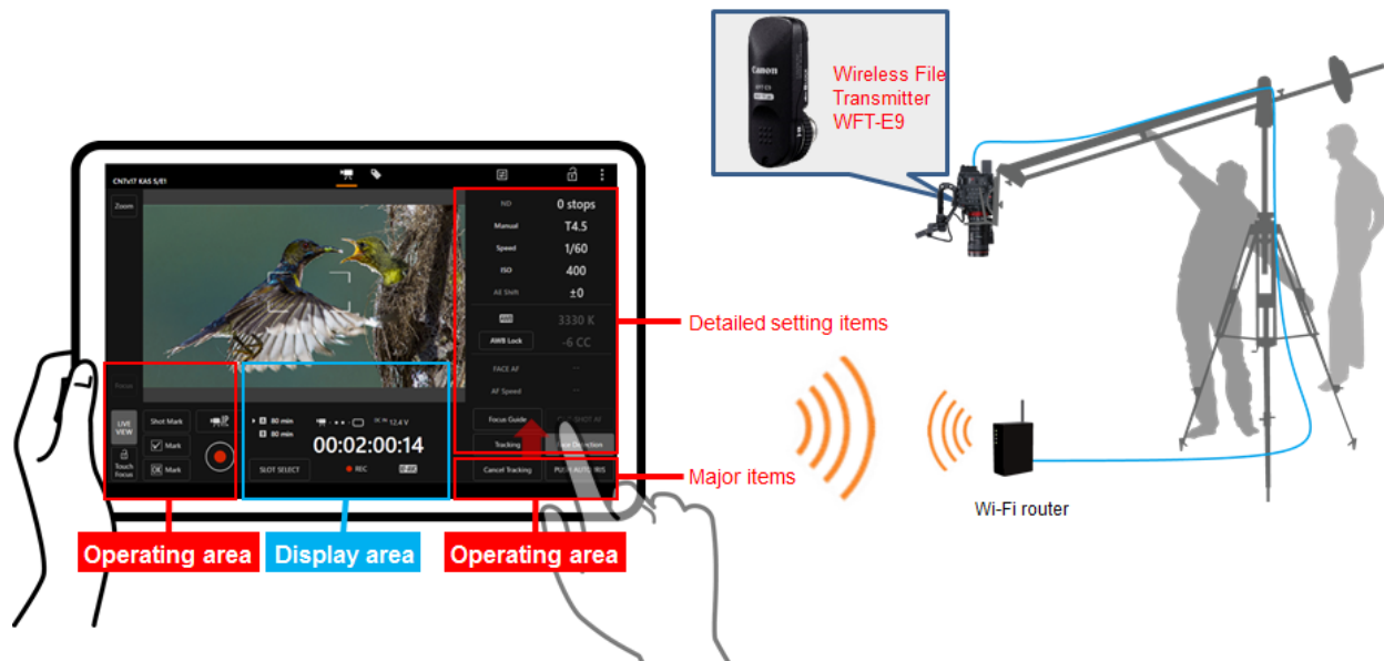
Figure 60 Browser Remote supports the control of the EOS C300 Mark III from a tablet
