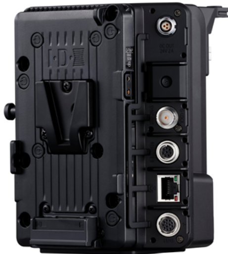
Figure 25 Outlining the connectivity that Expansion Unit 2 adds to the Base Model camera
