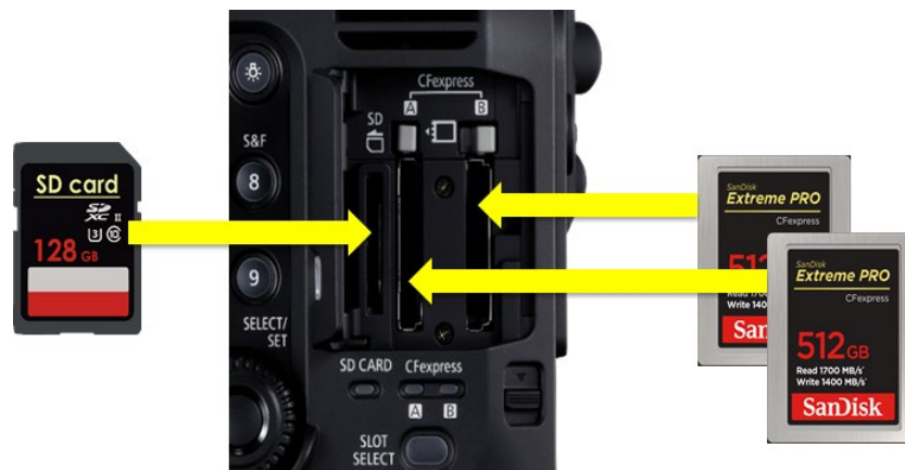
Figure 47 Two CFexpress 2.0 cards record the 4K Cinema RAW Light or the 4K XF-AVC file formats and an SD card records the Proxy video
