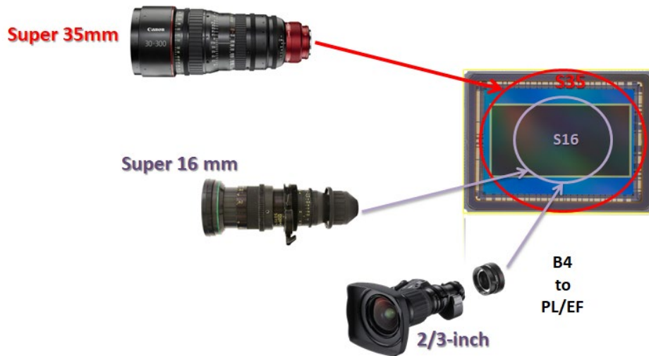
Figure 8 The Super 35mm EOS C300 Mark III can use S35 / S16mm cine formats and also broadcast lenses
