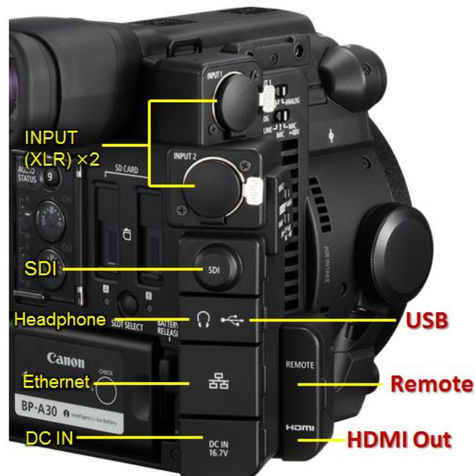
Figure 13 Showing the connectivity embodied in the EOS C200
