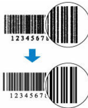
Printed Barcodes Are Not Recognized
