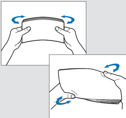
Take the stack of envelopes and loosen them, and then remove curling. Also remove the air inside the envelopes.
