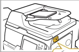
Insert a USB Flash Drive into the machine's USB port → place the original.
