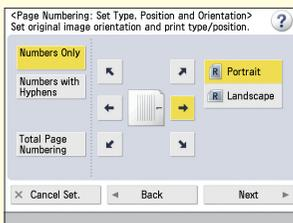
When setting page numbers or margins, take care with the orientation of the original. Select the button for an icon displayed on the touch panel in accordance with the actual orientation of the original you have placed.
