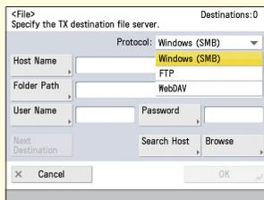
To send to a file server, it is necessary to set a server name (host name), folder path, user name, and password on the machine according to the settings of the server.
