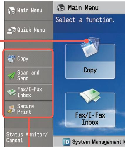
The first screen displayed after logging in to the machine is called the Main Menu screen. It includes buttons that lead to the various functions (function keys). The Main Menu screen can be freely customized by changing the number, layout, and background of the function keys and displaying a button for switching the language, etc.
