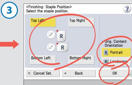
Select the position for stapling and the original orientation → press [OK].
