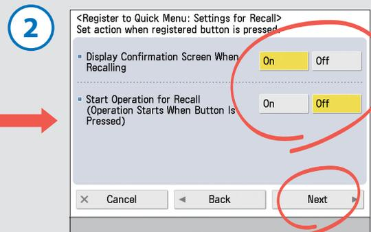
2 Confirm the settings → press [Next] → select the operation that will be performed when you press the registered button → press [Next].
