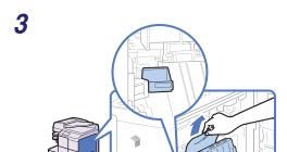
Pull down the upper cover of the fixing unit by the tab, and remove any jammed paper.
