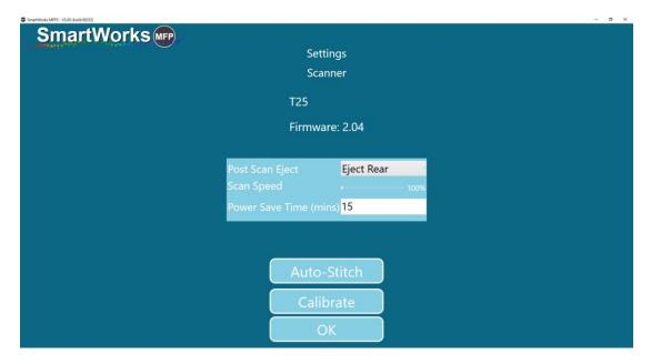
You can select whether the document is ejected out of the rear of the scanner after scanning (Batch mode will automatically use Eject Rear), or rewound to be ejected out of the front of the scanner.
