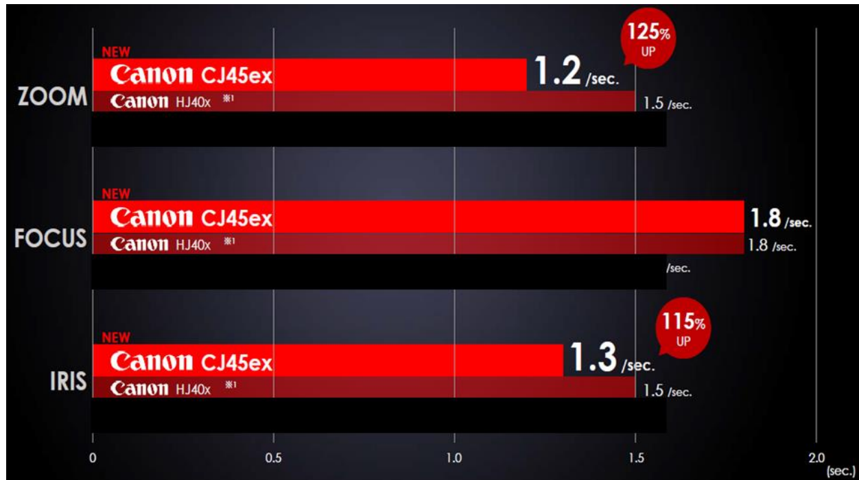
Figure 25 Outlines the speed performance of the digital drive unit for zoom, focus, and iris compared to those of the HDTV long zoom lens
