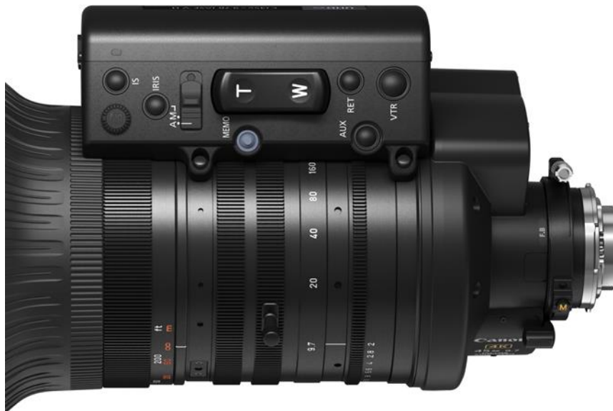
Figure 24 Close-up of the digital drive unit showing the physical engagement with the zoom, iris, and focus control rings and also showing the zoom control on the unit itself
