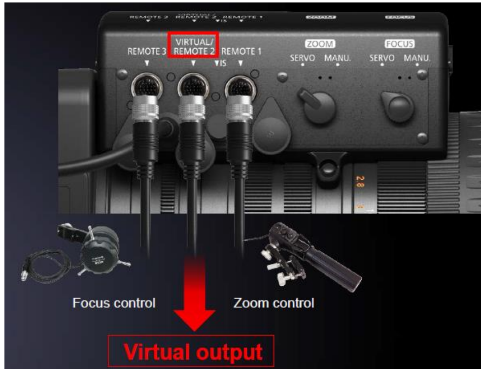
Figure 28 Remote 1 and 3 connectors are used for the standard broadcast zoom and focus controllers while Remote 2 delivers the digital data for virtual operations
