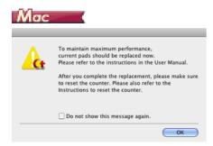
Furthermore, the counter in the scanner that records the number of pages fed also needs to be reset when you replace the rollers.
