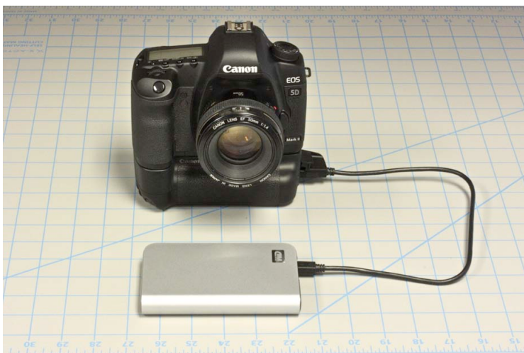
EOS 5D Mark II with Wireless File Transmitter WFT-E4A and 500GB external hard drive. Note that this drive would require its own power supply to work with the WFT-E4A.
