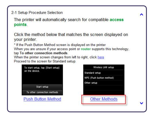
\*Note: If your printer's display looks like the screen shown above Push Button Method in the Setup Procedure Selection screen (2-1), tap To other connection methods before proceeding to the next instruction
