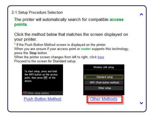
\*Note: If your printer's display looks like the screen shown above Push Button Method in the Setup Procedure Selection screen (2-1), press the Stop button on the printer before proceeding to the next instruction
