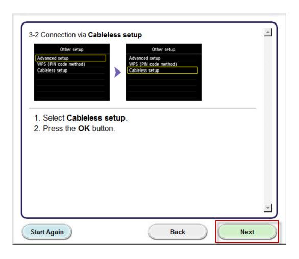
Press the **OK** button on your printer. When "Follow the instructions on the computer or smartphone...." appears on the printer's screen, click **Next** on the **Connection via Cableless setup** screen. (3-3).
