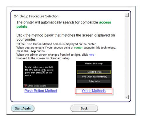
\*Note: If your printer's display looks like the screen shown above Push Button Method in the Setup Procedure Selection screen (2-1), press the Stop button before proceeding to the next instruction
