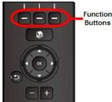
3. When finished entering the Network Key, press the Left function button (below **Done**)
