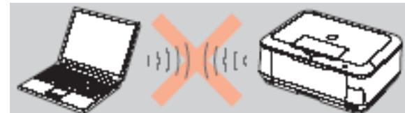
An "Ad-hoc connection," which establishes a direct connection to the computer over a wireless connection without using an access point, is not supported.
