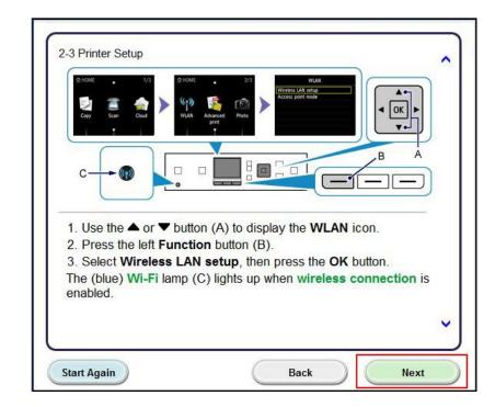
Continue to follow the on-screen instructions until the **Setup Procedure Selection** screen (3-1) appears. If your printer's LCD screen is the same as that shown above **Push Button Method** on the **Setup Procedure Selection** screen (3-1), press the printer's **Stop** button. Once your printer's screen is the same as that shown above **Other Methods**, click **Other Methods**.
