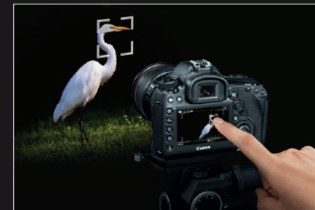
Dual Pixel CMOS AF with Touch AF enables easy subject tracking.
