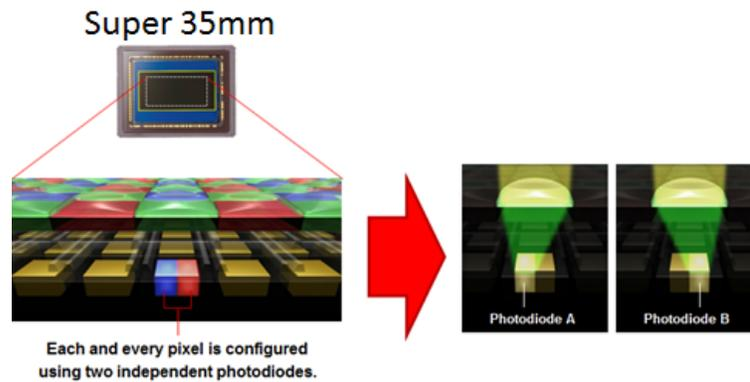
**Figure 4** A representation of the dual pixel CMOS image sensor with a specially designed microlens that optimizes the focusing of the incident light onto both photodiodes
