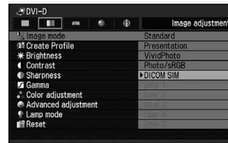
Press [OK] to select [DICOM SIM] and press the [MENU] button to exit from the menu screen. To check a test chart, press the [GAMMA] button when no menu screen is displayed.
