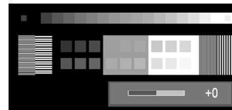
Press the [<] / [>] button to change the tone of the test chart. Make sure to select the tone in which all patterns are displayed.
