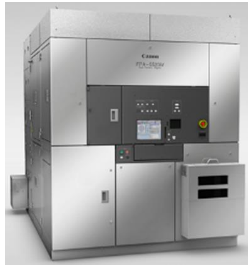
Figure 1. Figure 1. Canon FPA-5520iV i-line stepper
