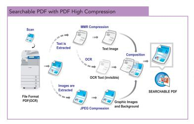
But now with Canon's new PDF Enhancement Kit for Universal Send, you can easily scan and convert documents into PDF files with text information included. This allows you to find scanned documents in a file server by keyword, and enables you to extract and reuse text data for creating a new document.
