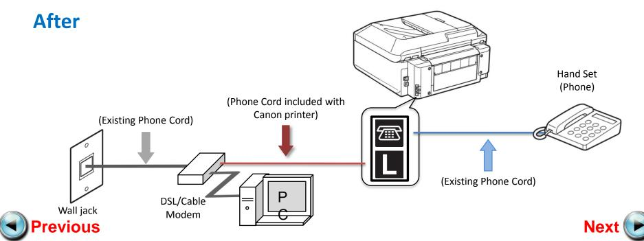
Plug the provided phone cord into the DSL/Cable Modem
