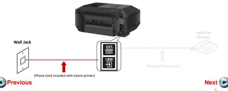
Plug the provided phone cord into the "LINE" jack located on the rear of the multifunction
