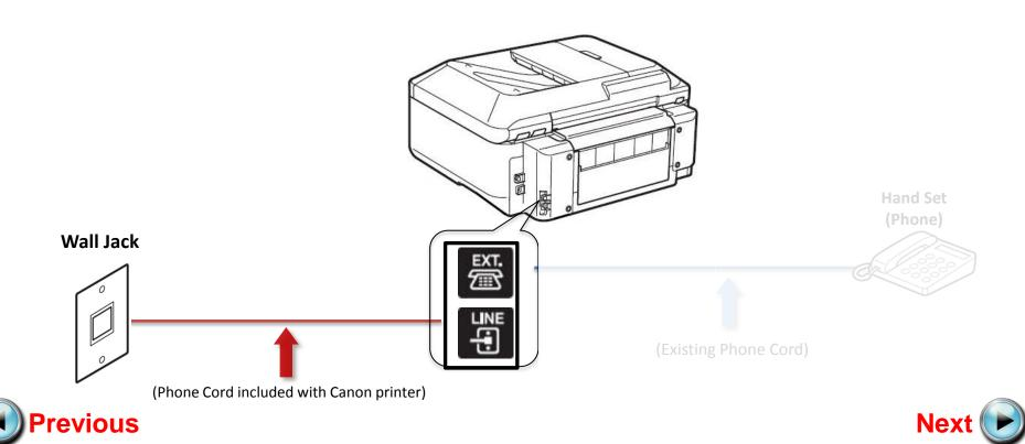
Plug the provided phone cord into the "LINE" jack located on the rear of the multifunction
