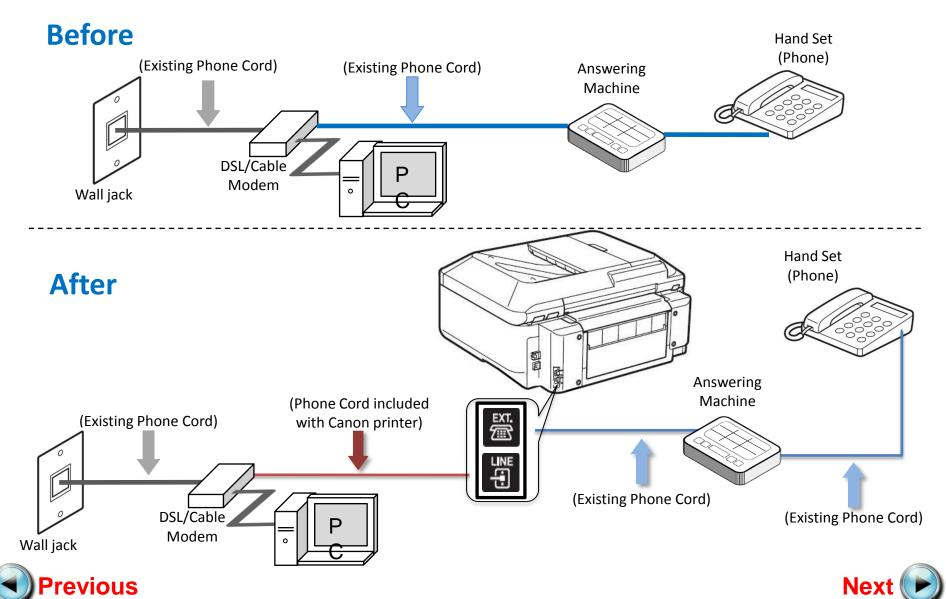
Plug the provided phone cord into the DSL/Cable Modem.
