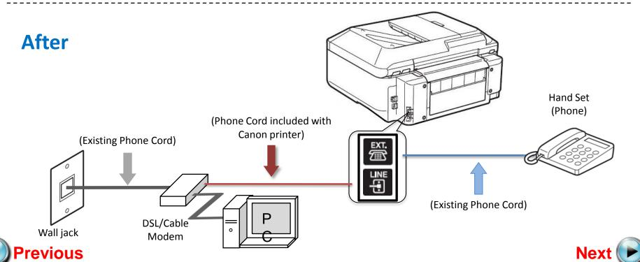
Plug the provided phone cord into the DSL/Cable Modem.
