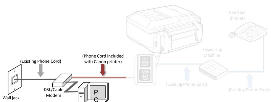
Plug the provided phone cord into the "LINE" jack located on the rear of the multifunction.
