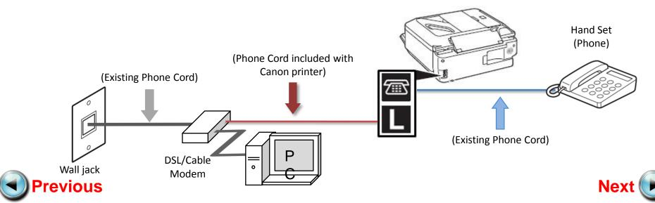
Plug the provided phone cord into the DSL/Cable Modem
