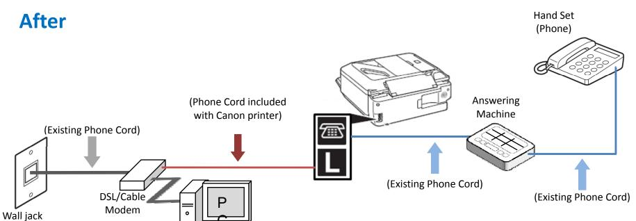
Plug the provided phone cord into the DSL/Cable Modem
