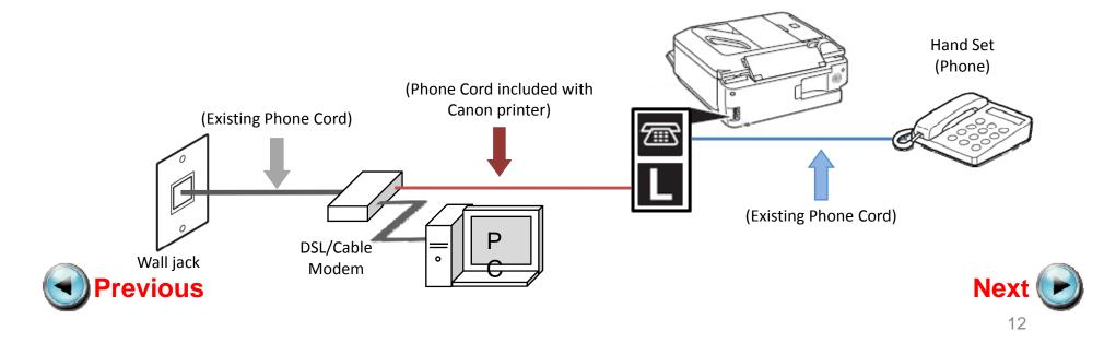
Plug the provided phone cord into the DSL/Cable Modem
