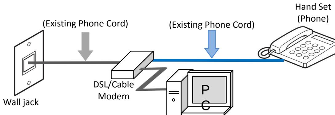
Setup Directions for DSL/Cable Modem Connection
