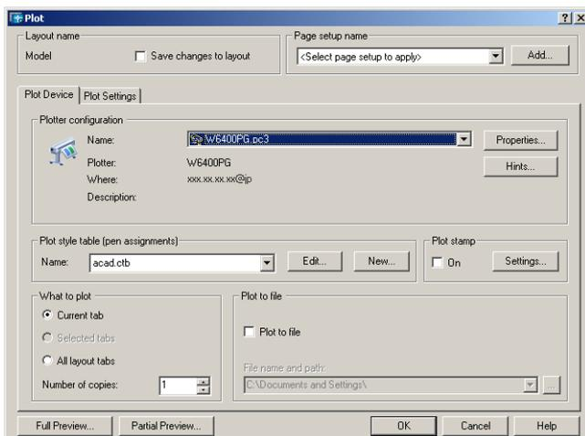
3. On the **Plot Device** sheet check the **Name** setting under **Plotter configuration** and confirm that **W6400PG** (the name of the printer you use) is displayed.
