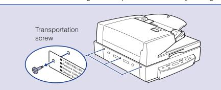
☐ Installing the Securing Braces
