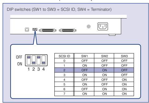
• When connecting the scanner and other SCSI devices in a daisy chain, make sure to set the terminator of the last connected SCSI device to ON, and set the terminator of all other SCSI devices to OFF.
