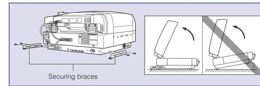
The scanner weights about 90.4 lb (41 kg). To lift or move the scanner, always use two people, one on each side. Never
