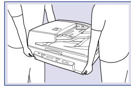
☐ When moving the scanner, make sure to secure the optical unit by installing the three transportation screws. For details, refer to "Installing the Transportation Screws" on page 5 of the Reference Guide.
