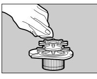
**3.** Carefully remove the lens from the lens unit and wipe the upper and lower surfaces of the lens with a clean dry cloth.
