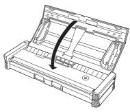
Push the section (front cover) at the front of the feed tray to close it.
