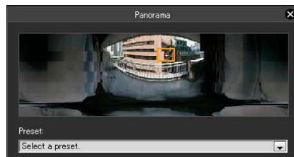
You can change the zoom ratio by dragging the yellow frame lines in the panorama window and changing the size of the frame. The zoom ratio will adjust to capture the area in the changed frame.
