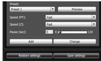
When [Preview] is clicked, the camera angle switches to this preset, and the new angle can be checked in the image display area.
