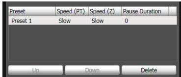
**3** Select a preset in the tour schedule list and set the pan, tilt, and zoom speeds using [Speed (PT)], [Speed (Z)], and [Pause (sec)], as well as the time in seconds during which the camera remains stationary at the preset position. Then, click [Change].
