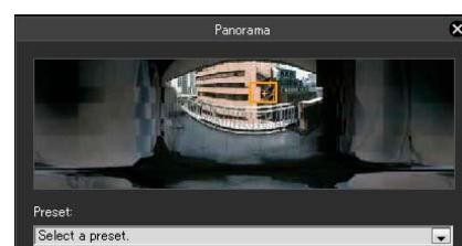
The frame lines within the display area show the image currently being captured by the camera.
