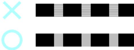
Test pattern B is printed for band adjustment.
