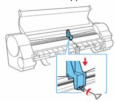
Attach the belt stopper that you removed and stored during the initial installation.
