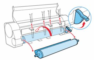
12 Lower the holder stopper lever, remove the stopper, remove the roll from the roll holder, then store the roll holder and the holder stopper.
