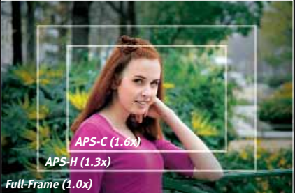
When using the same lens with different cameras, the angle-of-view varies depending on the sensor size.
