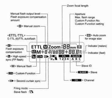
To illuminate the LCD panel, press the <:8:> button.
