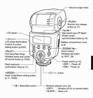
Asterisked buttons have a timer that keep the button's function active for 8 sec. ( 8) after you let go of the button. The < > illumination lasts for 12 sec.
