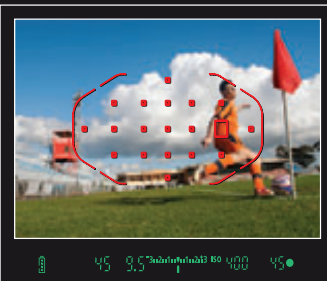
AI Servo AF tracking display — Provides instant feedback of AF points tracking a moving subject.
