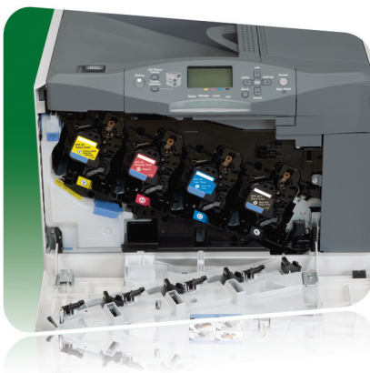
Front-load access to toner cartridges on LBP5460
