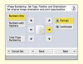
When setting page numbers or margins, take care with the orientation of the original. Select the button for an icon displayed on the touch panel display in accordance with the actual orientation of the original you have placed.
