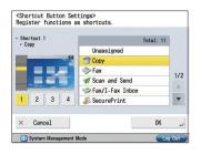
To delete a shortcut button that has been set, select [Unassigned] on the setting screen. The first screen displayed after logging in to the machine is called the Main Menu screen. It includes buttons that lead to the various functions (function keys). The Main Menu screen can be freely customized by changing the number, layout, and background of the function keys and displaying a button for switching the language, etc.
