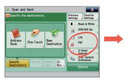
Press the file format button on the Scan and Send Basic Features screen.
