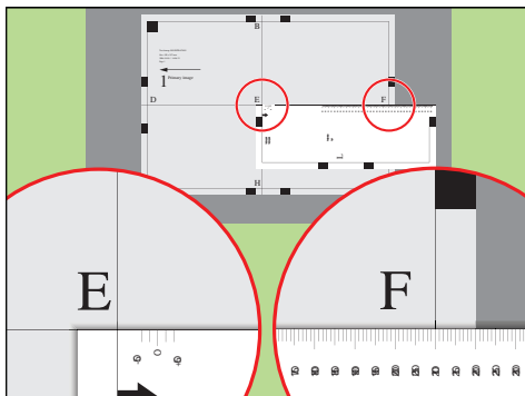
[34] Align the ruler with 'E' and read the value at 'F'
