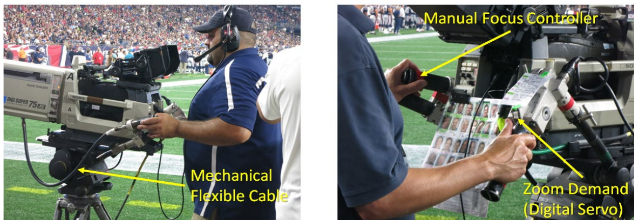
Figure 3 The Semi Servo control system comprises mechanical control of Focus and digital servo control of Zoom
