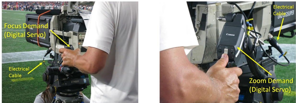
Figure 2 The Full Servo lens control system comprises digital servo control of both Zoom and Focus as shown
