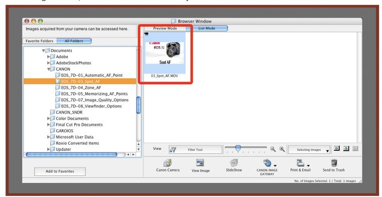
**Step 4:** Be sure that you use a freshly formatted memory card in the card reader. The video file and thumbnail can *only* be downloaded to a memory card by way of a card reader and through the ZoomBrowser/ImageBrpwser software application. With the memory card in the card reader, click on the video file in the ImageBrowser/ZoomBrowser window to make it active for writing the contents to the memory card.
